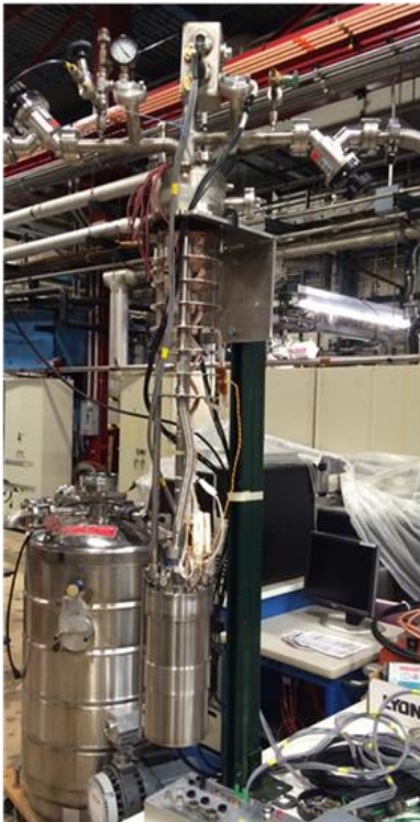
Insert into LHe dewar with cryo/vacuum and electrical connections
