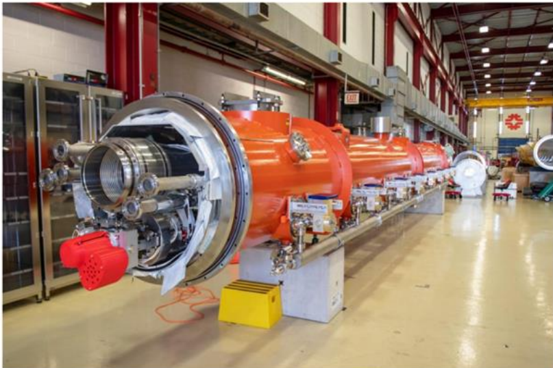
Fermilab 1.3 GHz CM for LCLS-II at SLAC
