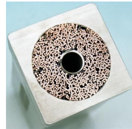
Cable in conduit cable (CICC) for fusion
