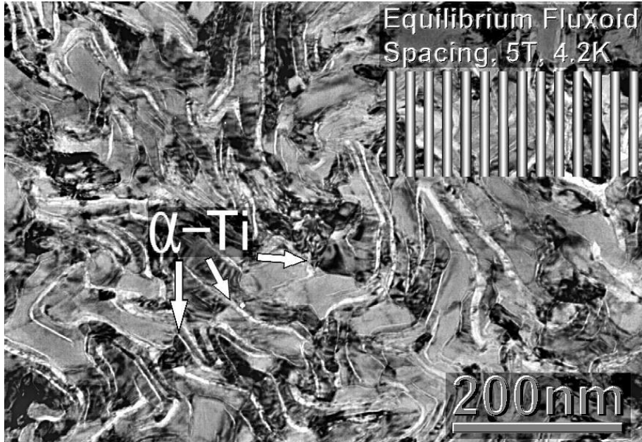
Microstructure of Nb-Ti
