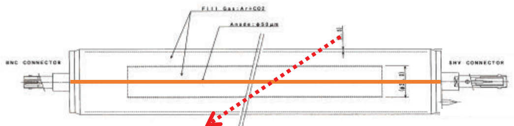
Anode Pt Wire, \phi 50\mu\text{m} (Gas: Ar+CO 2 )
