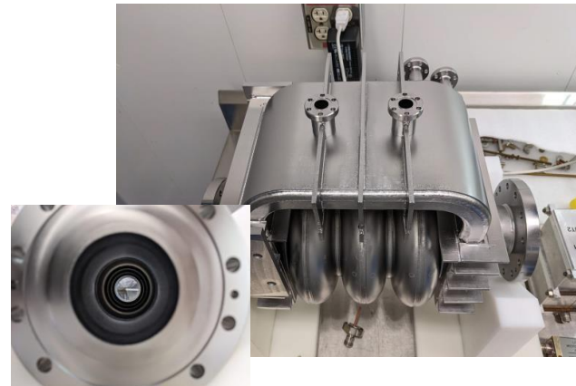
Cavity after 120um rotational BCP, 800C bake, external BCP to remove oxides
