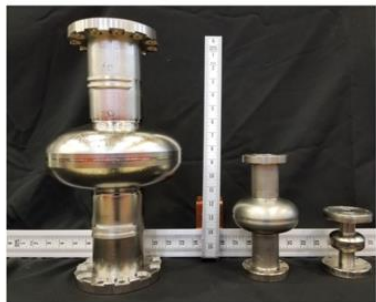
Fermilab SRF resonators
