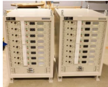
352 MHz solid-state amplifier modules @ APS
