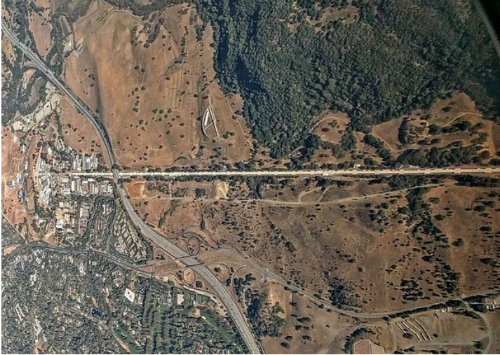
Stanford Linear Collider 2 miles, 100 GeV collision energy for e^+/e^-
