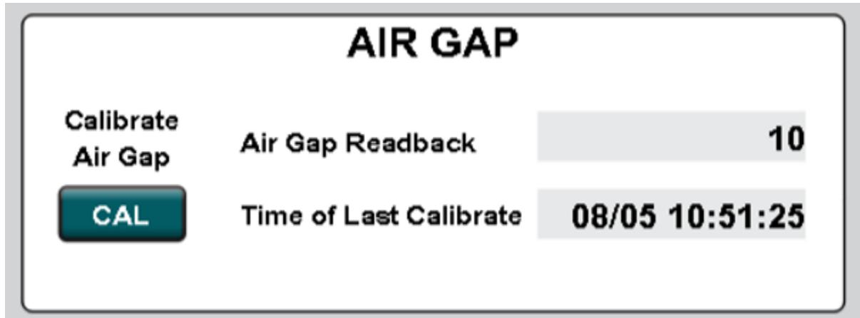
The calibration allows users to compute their device's offset distance on the stage. The offset distance refers to the difference of the stage Z coordinate and the Z-laser coordinate. The air gap distance is then calculated by the difference of the stage z coordinate and the offset, which is displayed on the PanelView. The following should be noted on the PanelView:
