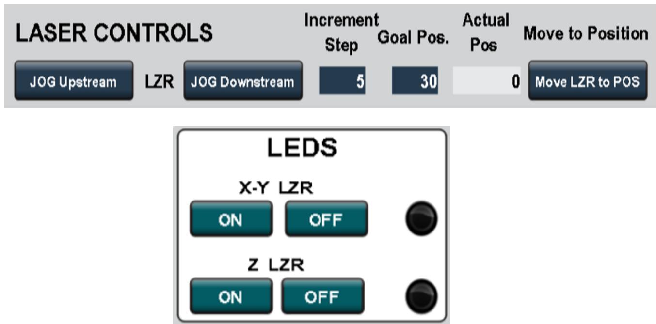
Users can control a laser crosshair system which assists with positioning devices in line with the beam. The Z laser position is defined as 0 at the beam exit and then increases as it moves further away from the exit. The values input are in units of millimeters.
