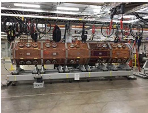
The radio frequency quadrupole (RFQ) was assembled and tuned in FRIB's linear accelerator tunnel. The RFQ prepares the beam for further acceleration in FRIB's superconducting linear accelerator.
