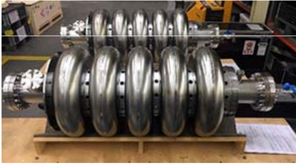
Two prototype superconducting cavities that could be used in an FRIB energy upgrade.
