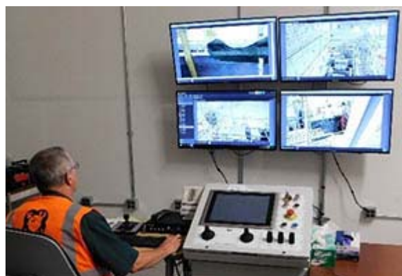
A new vision system will allow remote-handling operators to view and record work taking place. The operator is sitting next to a control unit that allows for remote operating of a crane. The crane uses guides to direct the magnet in and out of the beam-accelerating cryomodule ( for more about the crane, read this article ).
