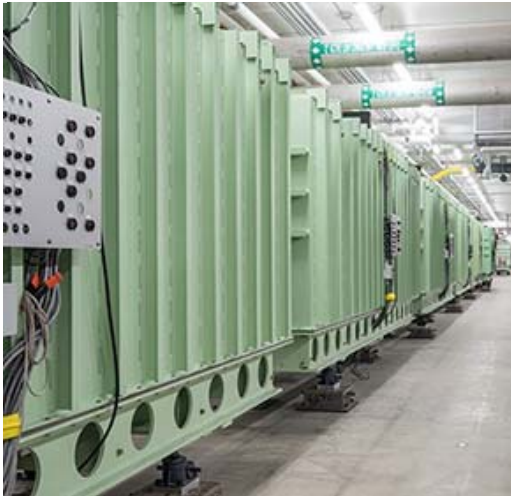
FRIB continues technical construction, and another significant milestone has been reached with all cryomodules now in production. Cryomodules are key components of FRIB's superconducting linear accelerator (linac). As of the end of March, 18 of 46 have been installed in the linac tunnel.
