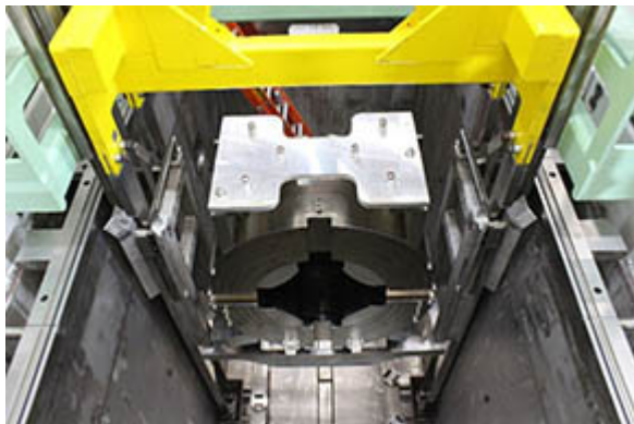
Using a remote-handling crane, a magnet is lowered into place during repeatability testing.
