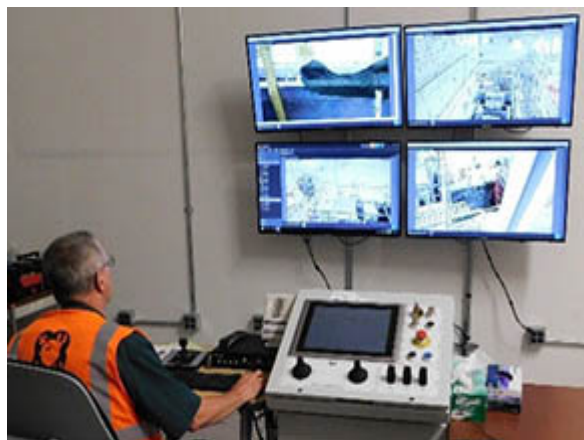
A new vision system will allow remote-handling operators to view and record work taking place. The operator is sitting next to a control unit that allows for remote operating of a crane. The crane uses guides to direct the magnet in and out of the beam-accelerating cryomodule (for more about the crane, read this article ).
