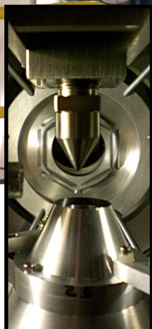
Above: A view of the JENSA system as installed in the ReA3 hall. Visible on the right is the dedicated beamline, with the target chamber, series of vacuum pumps, and the control panel. On the left is the industrial compressor, used to return the gas to the high pressures required to feed the jet. Left: A close-up photograph of the JENSA jet nozzle and gas receivers inside of the target chamber. Detector mounts are visible in the background.
