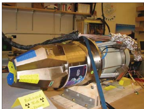
Top: An engineering drawing, based on the current GRETINA frame, of the 4\pi configuration of GRETA consisting of 30 of these modules. Above: A photograph of a GRETA quad module consisting of 4 HPGe capsules (6x6 segmented) closely packed in a common cryostat.
