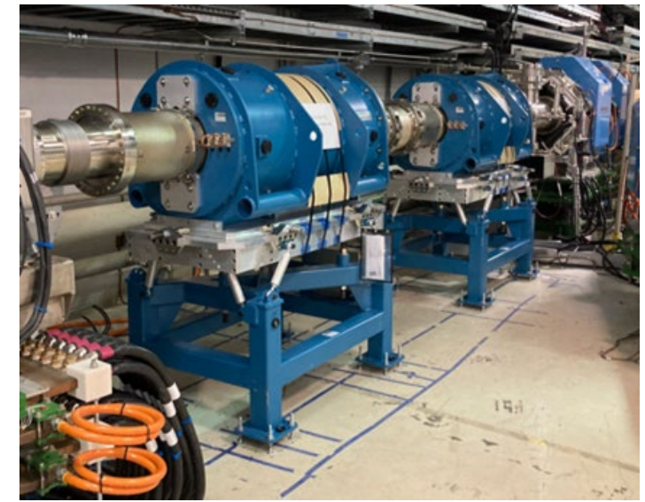
Two solenoids in the SNS ring for SCBD study
