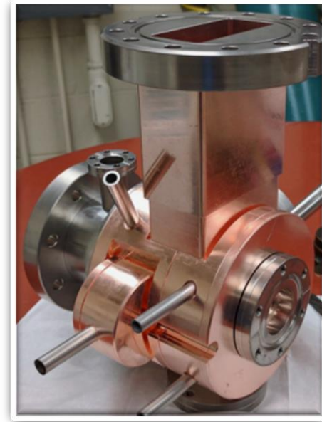
S-band Thermionic RF gun
