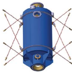
Figure 4.120: Helium vessel with hanging rod
