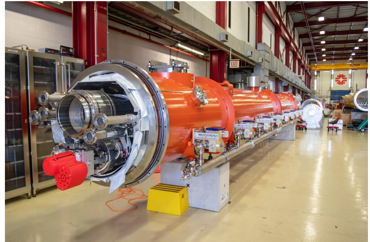
Fermilab 1.3 GHz CM for LCLS-II at SLAC
