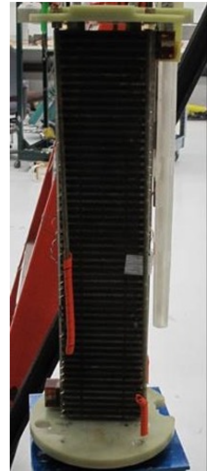
First half of Nb 3 Sn 0.5 m prototype after winding and reaction processes (left) and after epoxy impregnation and assembling the test set-up (right).
