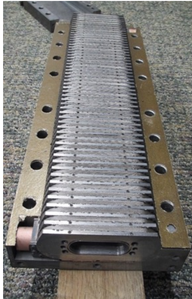
First half of Nb 3 Sn 0.5 m prototype after winding and reaction processes (left) and after epoxy impregnation and assembling the test set-up (right).
