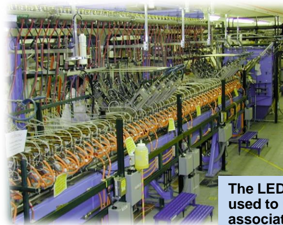
LEDA H + injector including LEBT (Low Energy Beam Transport)
