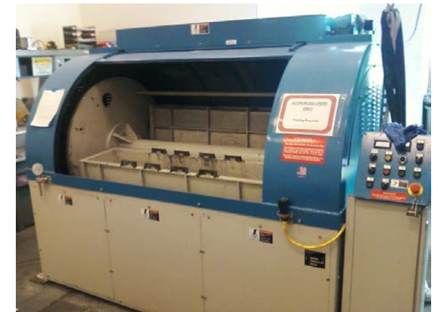
Barrel polishing machine at JLab SRF
