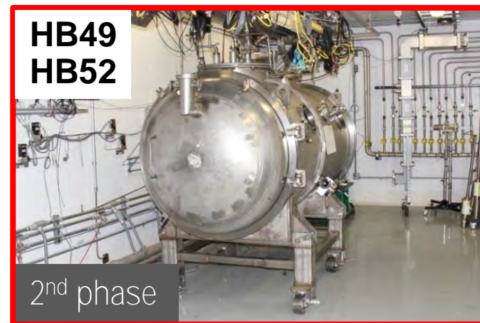
Processing of 6-cell cavity in HTA*
