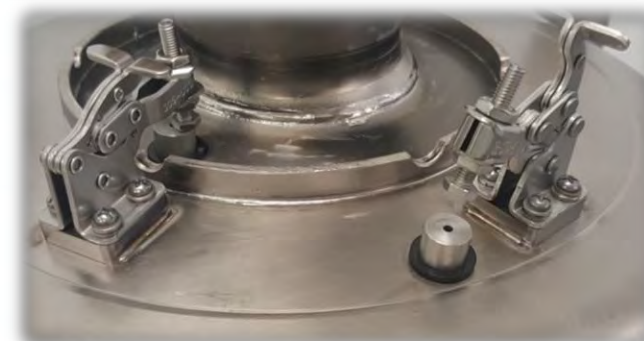
Single-cell cavity with small sample cut-outs.
