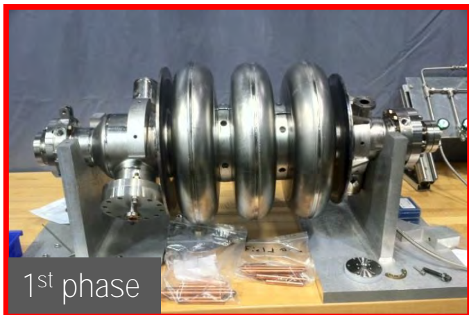
R&D with Nb samples and offline cavities
