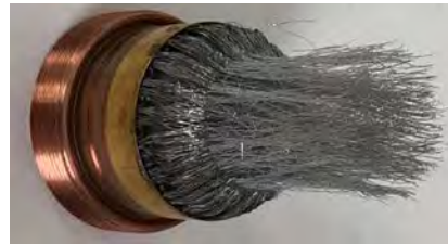
- eHD test cell with 960 Al cooling wires \blacktriangleright
