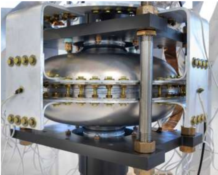
Conduction cooling setup: A ringed 650-MHz cavity attached to a cryocooler*.
