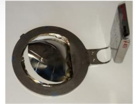
Burst disk rupture contaminates cryoplant
